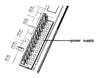
4. Position power supply connector P4 so the large tab on the connector faces the right side of the computer. Beginning with the six pins toward the back of the computer, carefully line up the holes in the connector with the pins in the socket. Make sure the holes fit over all six pins and then push in the connector.
